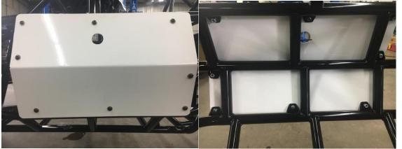
APPROVED FOR COMPETITION: INDIVIDUAL DOOR BAR CLAMPS/BOLT ON PLATE Minimum 1/8" (.125") thick magnetic steel intrusion plate measuring a minimum of 16" x 26". Intrusion plate must be bolted to a minimum of six (6) approved-design door bar clamps using the included 12 x 1/2" Allen button head bolts per the manufacturer's specification.
